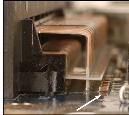
Figure 2. Filter capacitor very near to thru-hole connector.
